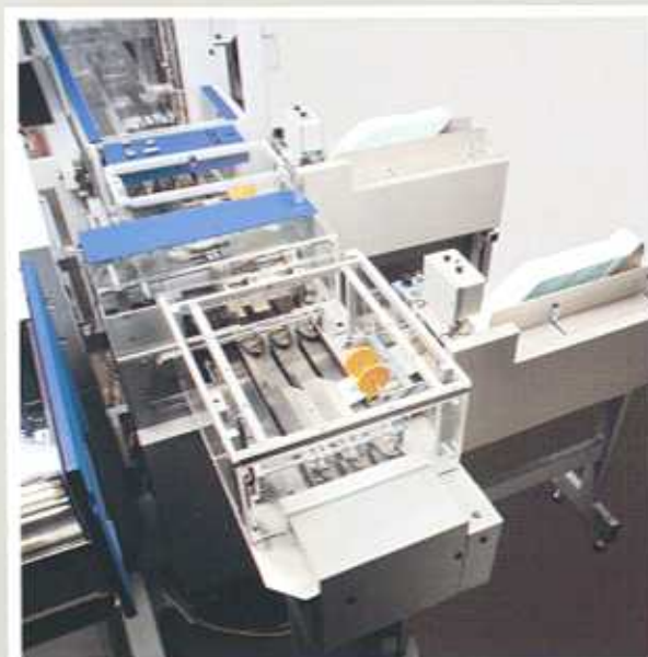
Collating track with single sheet feeders for feeding of front and back covers.
